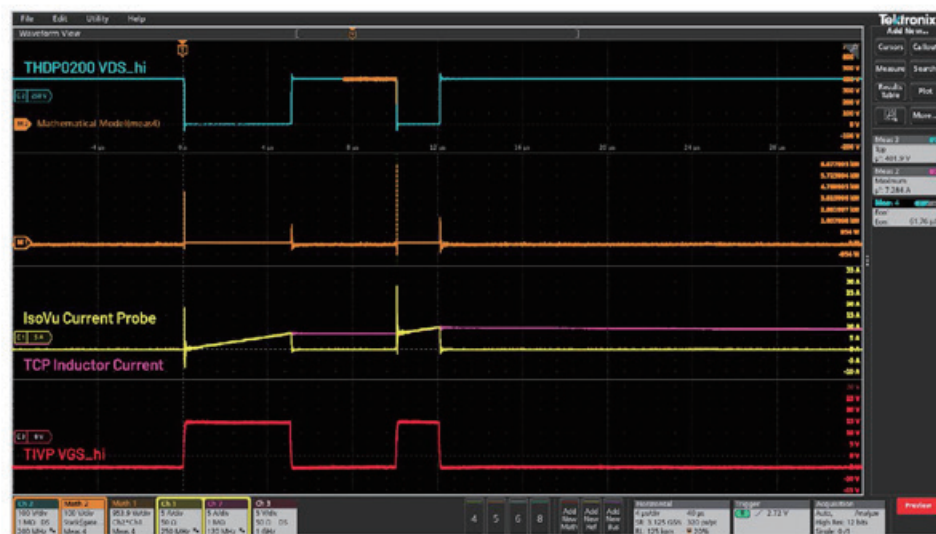
IsoVu Current probe clearly shows the ringing.
